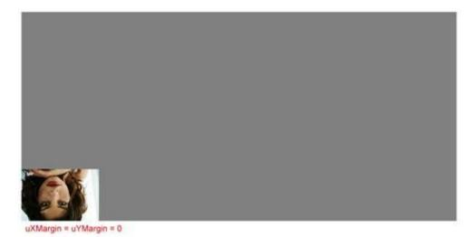
The image shows how the small job from Fiery XF prints on the table. To match this origin in Fiery XF, the origin of Fiery XF should be top right.
